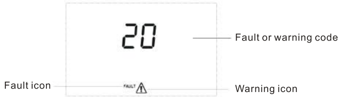
Figure 1-37 Fault and warning icons
