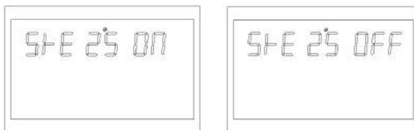
Figure 1-35 Inverter soft start setting page
