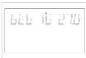
Figure 1-26 Setting of battery voltage point when mains switch back to battery mode
