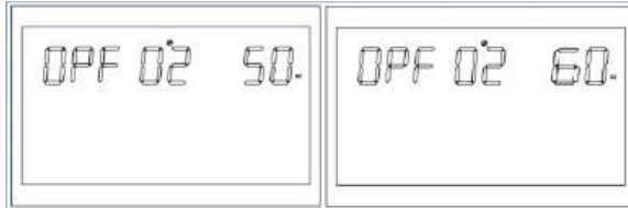
Figure 1-12 Output Frequency Setting Page
