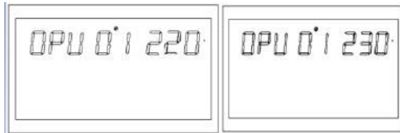
Figure 1-11 Output Voltage Setting
